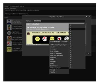
Next add a Halt Command and then a Wait Command for 5 seconds. The wait command can be adjusted for the desired effect. Then repeat the pattern starting with Drive To Trackmark A1, changing the CDE Decouple DLX number from the top number or using 0 every time, based on the consist, until all of the consist is accounted for. For our 3 wagons and a loco, we will Decouple 0 three times and our command sequence looks like this;
